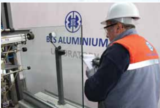
Horizontal Static Load Test
